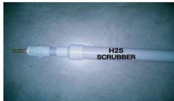
Fig 2 – H 2 S Scrubber
